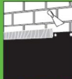
Alternatively, termination can be achieved by applying a layer of KSK Liquid Film or KOSTER Bitumen Mastic.
