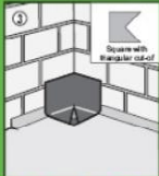
Place the prepared square freely (hand roller is recommended).
