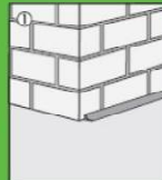
Before installation, place a flat of BIKUPLAN® KSK (Kaugelharter) concrete flat with RÜSTER Rapid Mortar.
