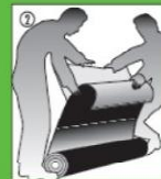
Peel back release paper 1m.
