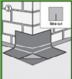
Place the prepared piece evenly and press freely (hand roller is recommended).
