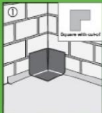
Place the prepared piece and press freely.
