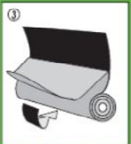
Stick exposed adhesive to substrate, follow the release paper back under the roll.
