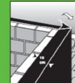
When appropriate BIKUPLAN® KSK should be fixed to the brick work, chamfer edges and corners beforehand to avoid puncture of the membrane.
