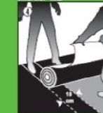
Adhere the membrane with 10 cm overlap.
