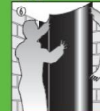
Place the membrane on top of the installed strip to the internal corner with minimum 10 cm overlap.
